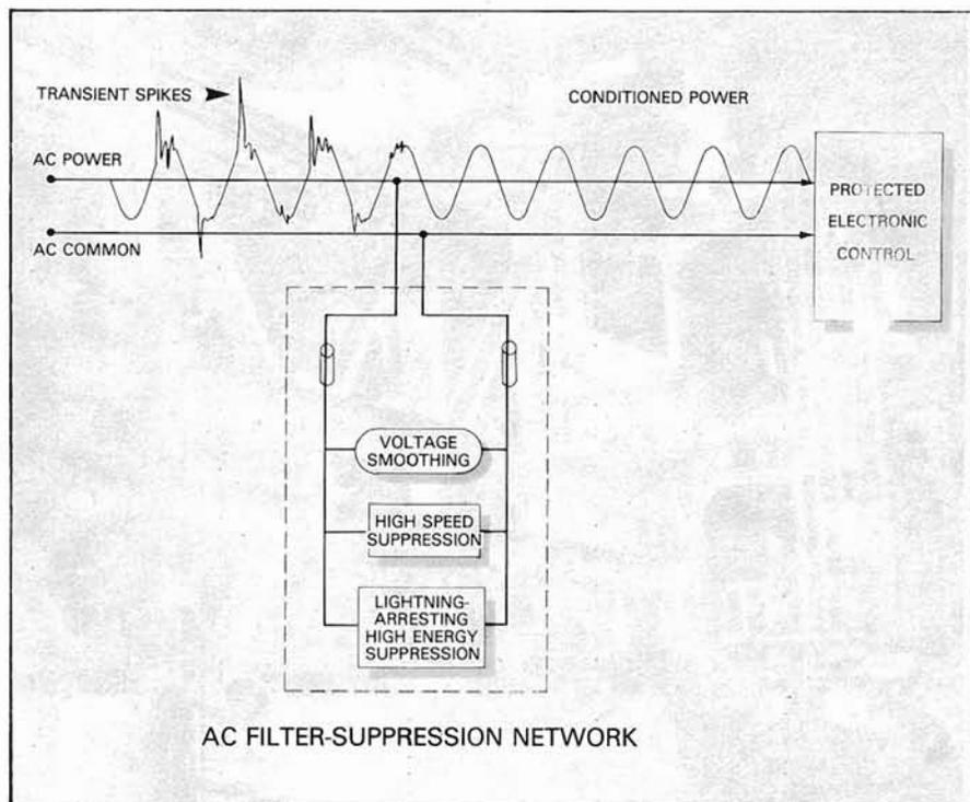
**3.** Process controllers, CAM computers and data loggers can suffer excessive downtime if not properly protected against harsh industrial AC power transients. Modern suppression networks can respond 10 to 1000 times faster to transients than older devices.
